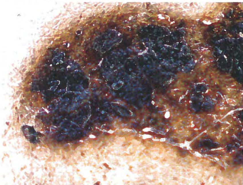
Fig. 76. Illustration of the effects of oak-gall tincture @ 200× enlargement – UB Leipzig, Cod. Lips. Gr. 16, f. 51r.
