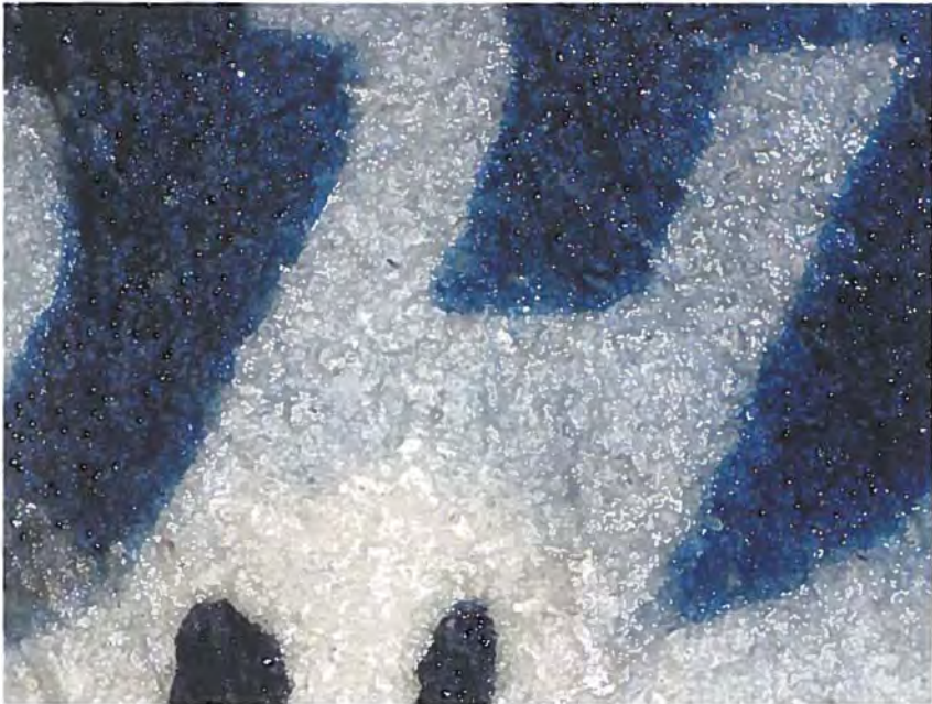
Fig. 83. Damage from Giobert tincture @ 50×enlargement – UB Leipzig, Cod. Lips. Gr. 2, f. XIr.
